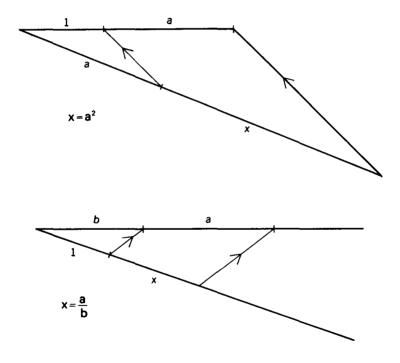
(2) Since b/a = 1/x, bx = a and x = a/b. To construct  $x = a^2/b$ , first construct a segment equal to  $a^2$ , then a segment equal to  $a^2/b$ .
