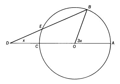
Let AOB be the given angle. Construct a circle with O as center and any convenient length as radius. Construct a line thru B intersecting diameter AC extended so that ED is equal to the radius of the circle. Then angle D is one-third of angle AOB.
