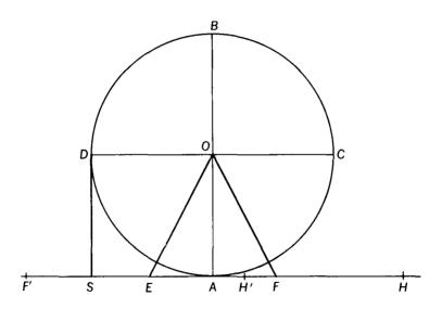
One method of constructing the regular polygon of 17 sides is as follows: In a circle of unit radius, construct two perpendicular diameters AB and CD. Let the tangents at A and D intersect at S. Divide AS into four equal parts, and let AE  $= \frac{1}{4}$ AS. Let the circle with center at E and radius OE cut AS
