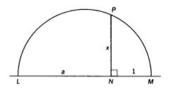
A semicircle is constructed on LM as a diameter. NP is perpendicular to LM (P is the intersection of the perpendicular and the semicircle). Then  $x = \sqrt{a}$ .
