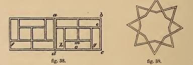
EXAMPLE 32, fig. 39, is described by somewhat the same method as figs. 30, 31, the points, as e, being joined by straight lines in place of arcs of circles. The method of drawing the ornament in
