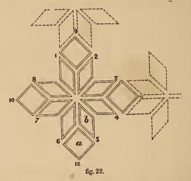
to the diagonal lines c b, a d, draw lines equal to i i. From e, one end of the octagon side, draw a line perpendicular to c d, joining the diagonal a d in h. From n, the end of another side of the octagon, draw parallel to c d a line cutting the diagonal d a in o, parallel to e h, k t; draw lines p t, n s; two of the rhomboids will thus be formed; the remainder are drawn in a similar way. These being obtained, the squares, as in fig. 22, are easily drawn.
