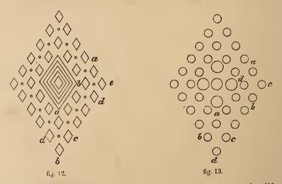
EXAMPLE 11, fig. 13, are illustrative of a "diaper" pattern, the different parts of the pattern forming a series of diamonds, as a, b, c, d. The method of drawing EXAMPLE 12, fig. 14, is shown in fig. 15. The application of this to .he delineation of a Gothic perforated parapet is shown in
