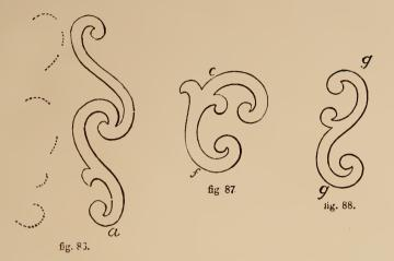
**EXAMPLE** 59, fig. 89. One half of an elegant scroll, well adapted for a wall-paper pattern, may be constructed as follows :—To the part a, fig.
