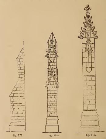
In fig. 177 we give an illustration of an Early English buttress; in fig. 178 one of the "Decorated;" and in fig. 179 one of the "Perpendicular."
