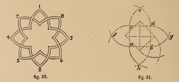
are formed in like manner, the centres of the arcs being found in a square drawn diagonally in the first, as shown in fig. 31. The ornaments
