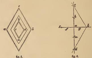
EXAMPLE 4, fig. 5, is the "lozenge" or diamond shape. Fig. 6 shows the manner in which it is drawn: two lines, c b, e d intersect, at a; a c,
