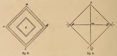
take half of c d, fig. 3, as c e, and set it off from m, fig. 4, to e, h, g, f; join these, and parallel to them draw the internal squares.
