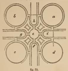
diagonal square, the side of which is equal to gh; the centre e is at the intersection of the two diagonals of the larger square, as ac, bd. These points being obtained, the remainder of the figure, and its repetition to any extent desired may be easily drawn.
