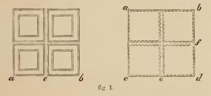
tile design. The diagram to the left shows the manner of drawing this: a series of squares are formed in lines distant from each other, as at e or f, the side of each square being df.
