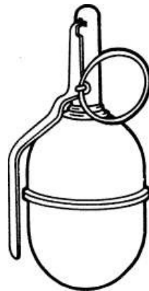
Figure U-9. Chinese Communist type 59 defensive hand grenade.
