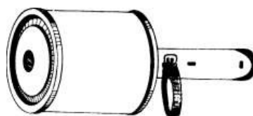
Figure 4-15. Fragmentation explosive device. AGO 718A
